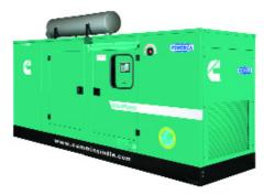
The acoustic enclosure is made of 1.6 mm thick CRCA sheets in Munsel green shade and a structural/ sheet metal base frame painted in black. The walls of the enclosure are insulated with fire retardant foam so as to comply with the 75 dBA at 1 mtr sound levels specified by Ministry of Environment & Forest.
